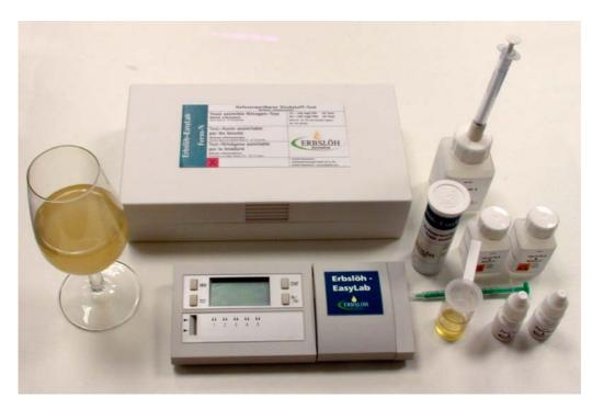
Easy-to-handle rapid test to determine analytical parameters required for process control in grape must and wine:
